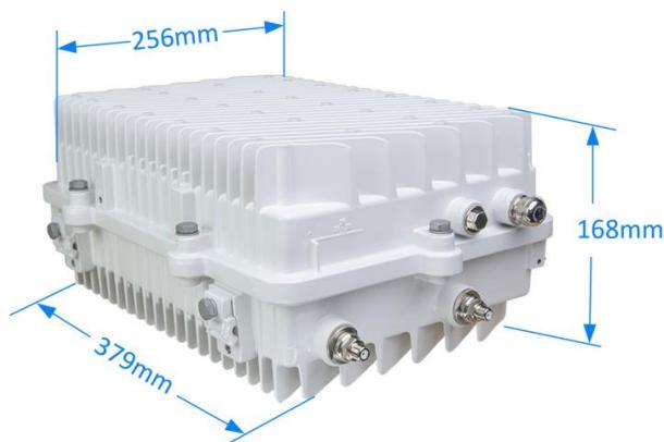
CC8800-Hybrid is mainly composed of DOCSIS and R-OLT module, power module and RF module, and the external interface description is shown in the below.
