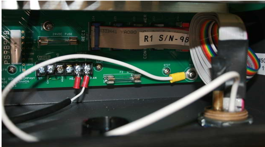
Figure 23 : Transducer Connection Inside KA98002 Transceiver Unit
