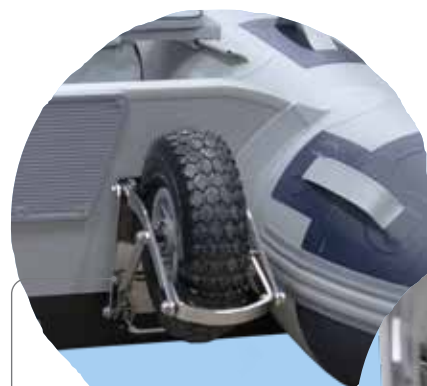
Quick release to remove wheels
