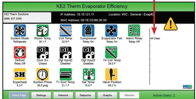
If the controller is connected to the Internet, the KE2 Evap OEM can also send text messages and/or e-mails to immediately notify all necessary personnel of the alarm condition.
