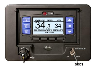
To stop the unit, place the START/RUN-OFF switch in the OFF position. The refrigeration system and engine will shut down immediately while the control system completes a shut down sequence, and then the display will go blank.
