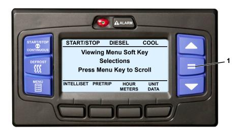
2. Press the MENU key until INTELLISET is displayed. Then, press the INTELLISET soft key to display the IntelliSet screen.
