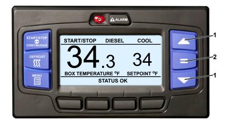
With the system powered up (START/RUN-OFF switch in the START/RUN position) and the default screen displayed (press the BACK or EXIT soft key if required), press the ▲ or ▼ key to bring the displayed setpoint to the desired value.
