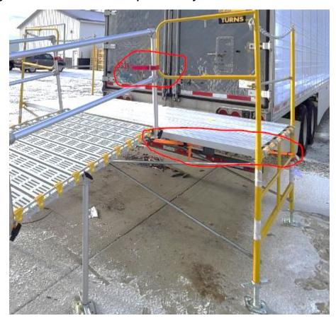
When loading or unloading the trailer, use the provided portable secondary ramp. You will not be able to shut the trailer doors when this ramp is in place, so it is important to only install when actively loading or unloading. When not loading/unloading, remove the portable ramp and fully shut and secure the rear trailer doors to prevent cold air from escaping:
