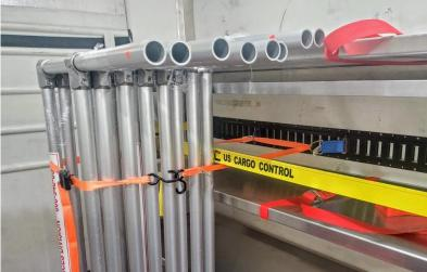
Loosen and remove all ramp legs, place legs, hand screws and rectangular machined nuts into storage crate.
