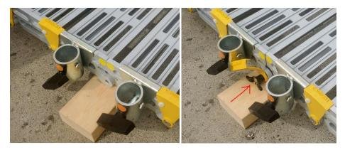
Using at least two and up to four people, lift the trailer side end of ramp and drag the ramp towards the trailer into position with ramp upper end plate placed over the rear-most lip of the trailer, as shown in photo. Make sure that ramp is positioned 90-degrees to trailer and properly positioned on tail of trailer.
