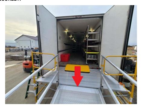
Position two (2) heavy-duty ratchet straps so that they attach to the uppermost ramp legs, run underneath the scaffold platform, and then attach to the rear bumper of the trailer. Adjust and ratchet down until tight and fully secured
