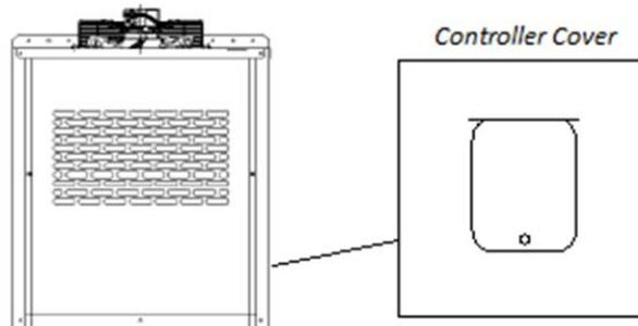
3. Turn the rocker switch under the controller (led display) on. Note: When power is applied, display may be on but if the rocker switch is not on, the unit will not operate.
