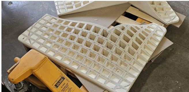
Waffle forms: ribs cut, assembled, then milled to shape.
