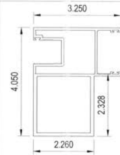
10 HEAVY LOCK STILE 113-017 TYP. WALL THK = 0.090" MAT: ALUM. ALLOY 6063-T6
