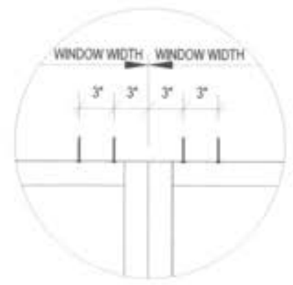
DETAIL "A" TYPICAL CLUSTER OF ANCHORS AT INTERLOCKS TOP & BOTTOM (ONLY AT UNCLIPPED MULLION CONDITION)
