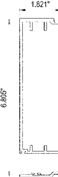
11 HEAVY MALE VERTICAL MULLION 101-411 TYP. WALL THK = 0.125" ALUM. ALLOY 6063-T6
