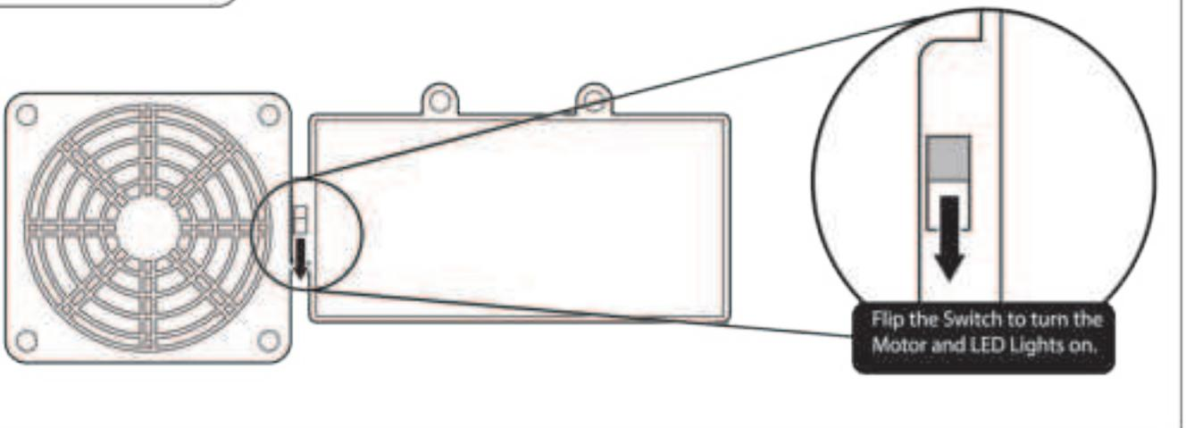
Flip the Switch to turn the Motor and LED Lights on.
