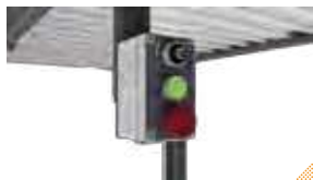
Key switch for each operation with emergency stop button
