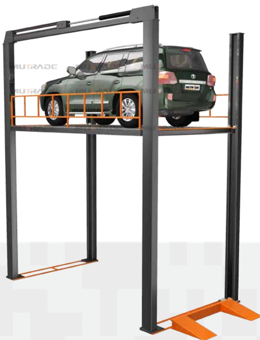
FP-VRC is simplified car elevator of four post type, able to transport a vehicle or goods from one floor to another. It is hydraulic driven, piston travel can be customized according to actual floor distance. Ideally, FP-VRC requires an installation pit of 200mm deep, but it can also stand directly on ground when pit is not possible. Multiple safety devices make FP-VRC sufficiently safe to carry a vehicle, but NO passengers at all conditions. Operation panel can be available on each floor.
