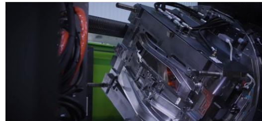
Integrated CANNON dosing unit for PUR
