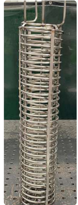
Welded double coil unit for medicine manufacturing machinery (circular tube, stainless steel 316L, ¼" x 0.035")
