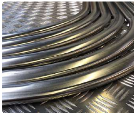
Marine handrail (oval tube, stainless steel 316L, 39.5 x 20.5 x 2mm)
