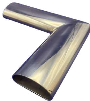
Balcony railing corner (D-shaped tube, 65 x 28 x 2mm, stainless steel 316L, mitre-cut then welded without connector)
