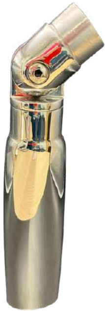
Oval tube with ends formed to 33.7mm OD to fit standard handrail bracket (stainless steel 316L, 61 x 37 x 2mm)
