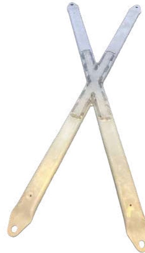
Welded and pressed car interior support brace (flat-sided oval tube, aluminium 6060 T6, 36 x 13.5 x 1.5mm)
