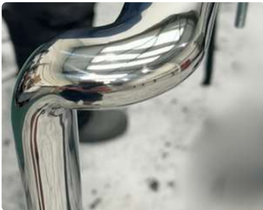
Yacht balustrade (oval tube, stainless steel 316L, 47 x 25 x 1.5mm with A and B Plane connectors, mitre-cut at 45° then welded to form a compound curve)
