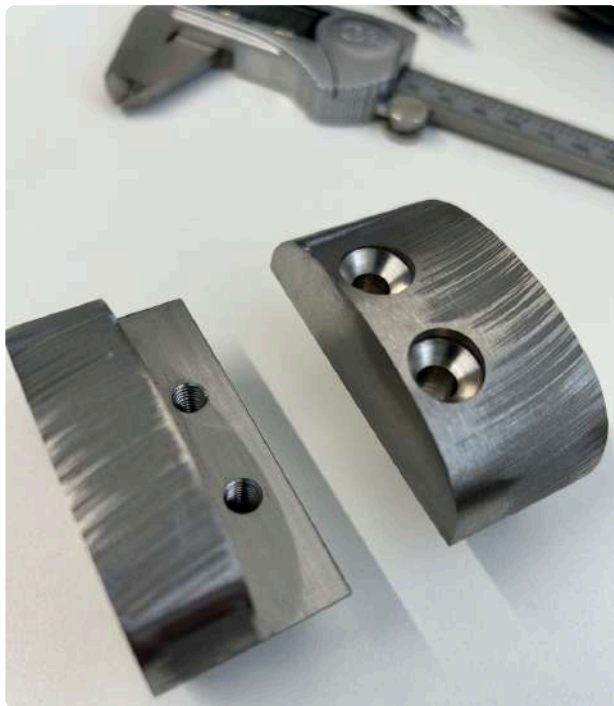
CNC-machined lap joint for oval tube assembly (oval tube, stainless steel 316L, 61 x 37mm)
