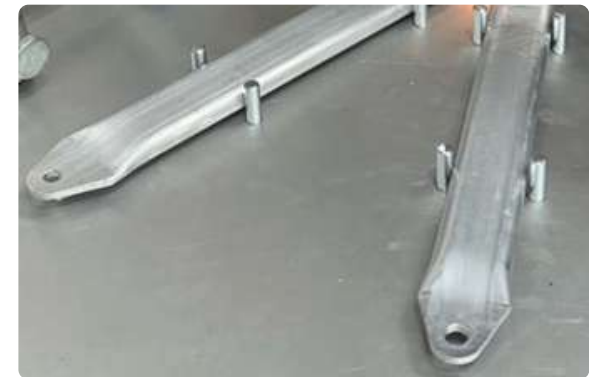
Welded and pressed car interior support brace (flat-sided oval tube, aluminium 6060 T6, 36 x 13.5 x 1.5mm)
