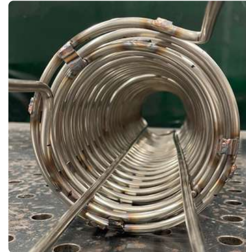
Welded double coil unit for medicine manufacturing machinery (circular tube, stainless steel 316L, ¼" x 0.035")
