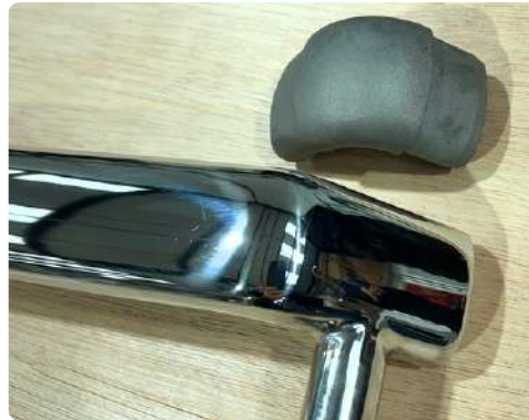
Yacht balustrade (oval tube, stainless steel 316L, 47 x 25 x 1.5mm with A Plane elbow connector, mitre-cut at 45° then welded and polished)
