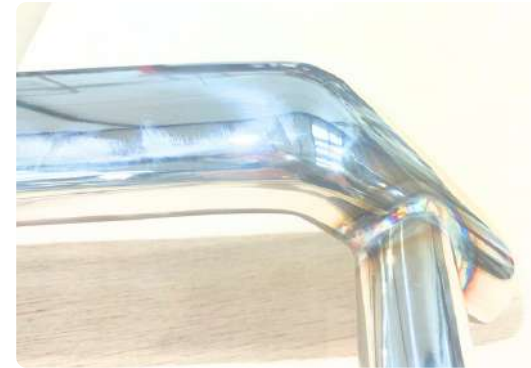
Yacht balustrade (oval tube, stainless steel 316L, 47 x 25 x 1.5mm with A Plane elbow connector, mitre-cut at 45° then welded and polished)
