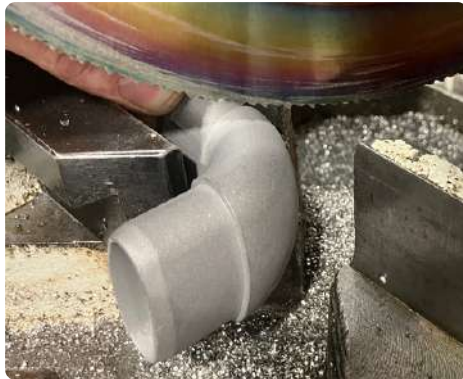
Yacht balustrade (oval tube, stainless steel 316L, 47 x 25 x 1.5mm with A Plane elbow connector, mitre-cut at 45° then welded and polished)
