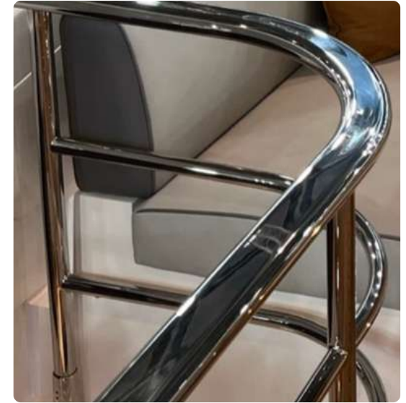
Yacht grab rail (flat-sided oval tube, stainless steel 316L, 62 x 31 x 2mm)
