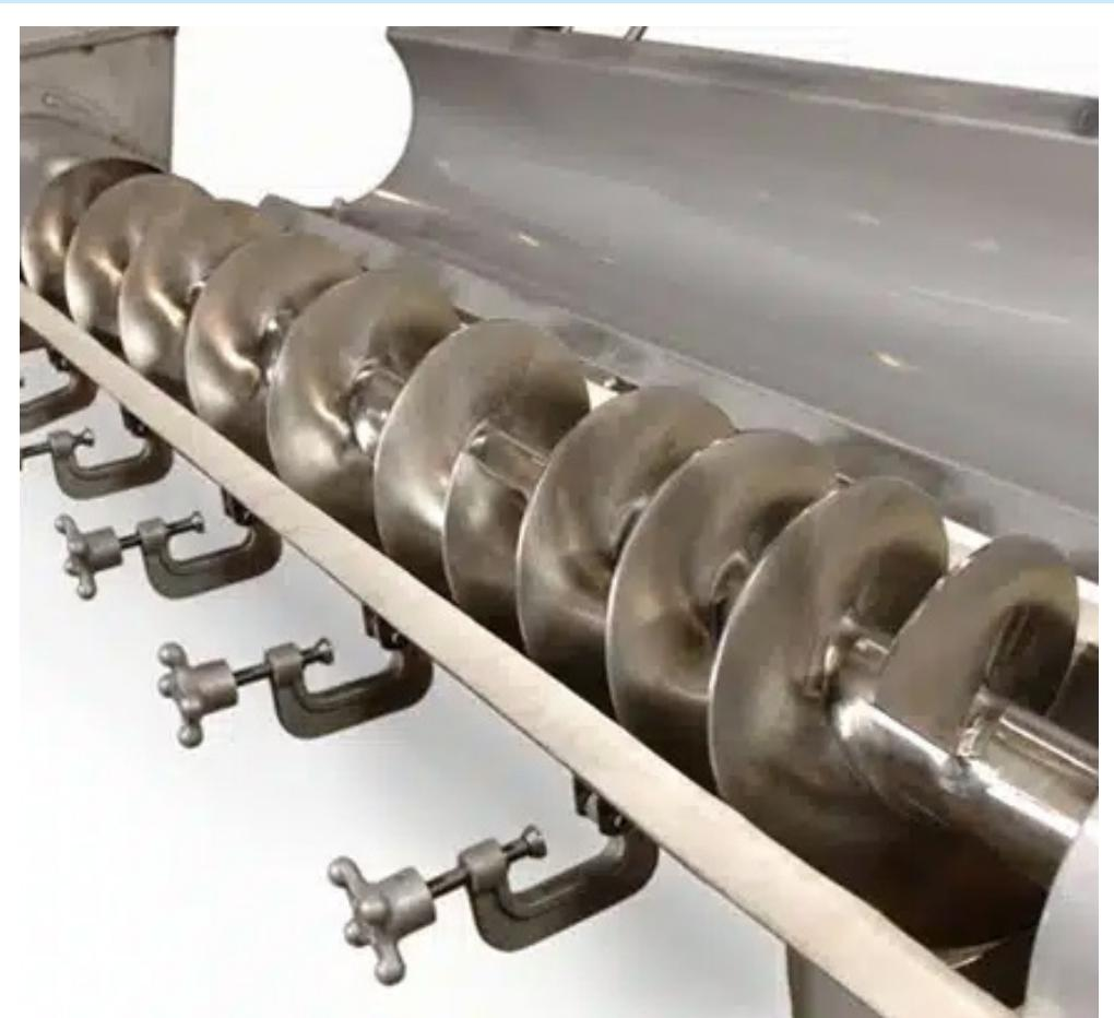
This case study details the design and implementation of a horizontal and vertical screw conveyor system to reliably and hygienically transport granulated sugar into a sugar liquifying tank for an ingredient supply company. The manufacturer needed to replace its antiquated process, which posed contamination risks, created dust, and was constantly breaking down.
