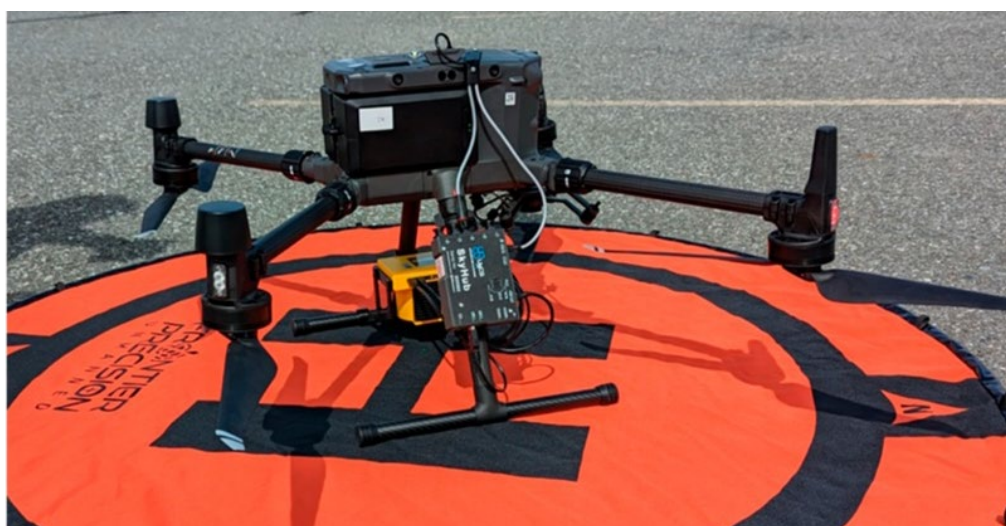
Figure 1. Hardware components of the methane survey system, excluding the UgCS software.
