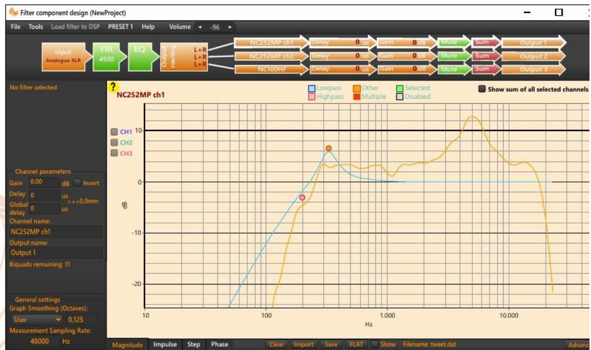
Picture 32: Graphical filter design screen
