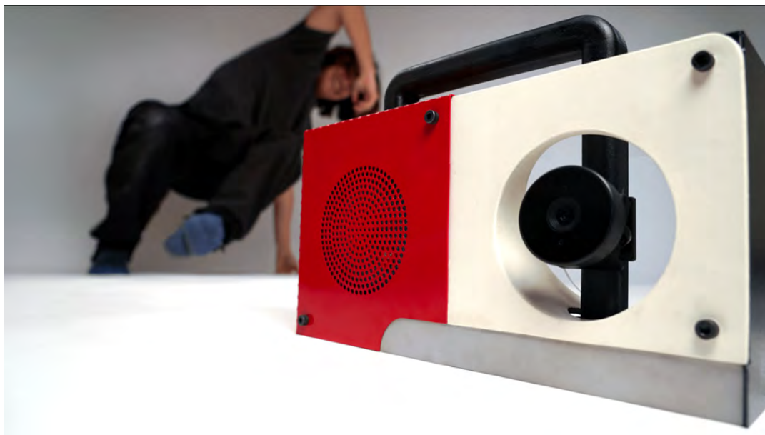
Figure 1: Be the Beat is an interactive boombox that takes dance videos as input through the camera and outputs matching music. The device allows freestyle dancers to guide the quality of music and discover new choreographies.
