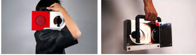
(a) Boombox Front View. The model is holding Be the Beat on their shoulder, showing the camera in the right cutout with a handle extending through the body. (b) Boombox Back View. The clear acrylic back allows the user to see the internals. This shows all the connecting screws and the handle geometry.
