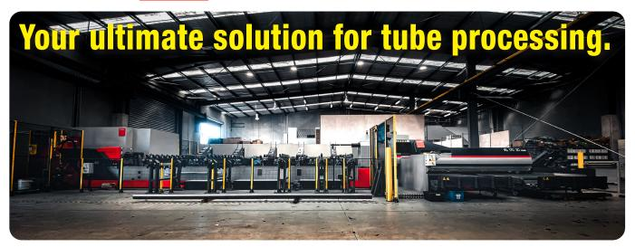
We are very excited about our new piece of kit, the Bystronic FL170 Tube Laser, which combines the unique benefits of fiber laser technology with the versatility of 3D cutting.
