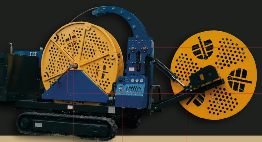
**COIL INJECTION HEAD 2,000 LB** DOWNWARD FEED FORCE
