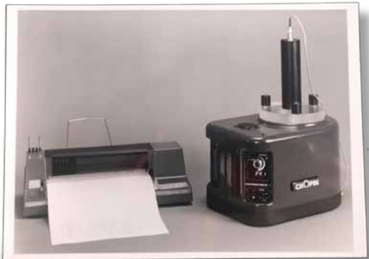
The original Rheo (Rheofermentometer) for measuring dough during proofing.
