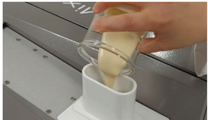
Liquid batter entering the Mixolab 300 for analysis.
