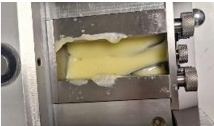
Mixolab 300 used for mozzarella cheese melting tests.
