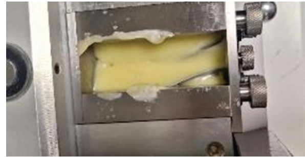
Mixolab 300 used for mozzarella cheese melting tests.
