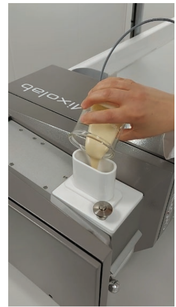
Mixolab 300 includes a novel dough introduction design for analyzing all types of dough consistencies including, sticky doughs, crumbly doughs, and batters.
