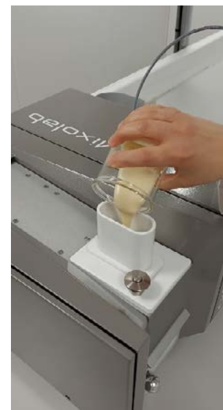
Mixolab 300 includes a novel dough introduction design for analyzing all types of dough consistencies including, sticky doughs, crumbly doughs, and batters.
