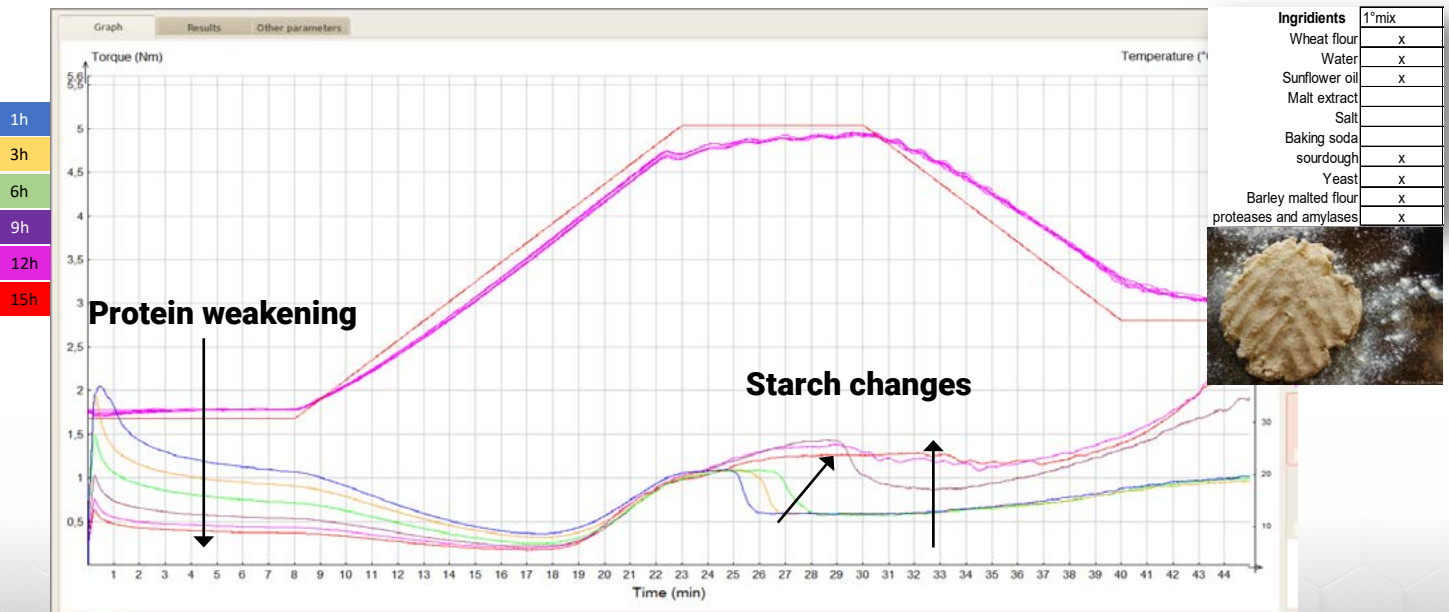
As this example "Full" Dough Test of a cracker dough indicates, dough consistency can change significantly over time.
