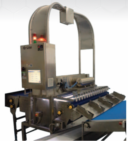
Q-Bake™ Vision Inspection for baking.
