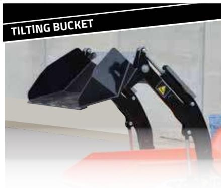
The tilting bucket not only load the dumper but can unload it frontally
