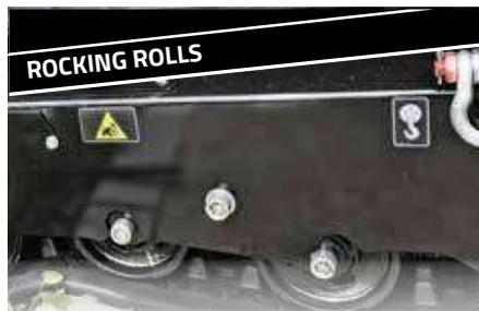
The machine's undercarriage oscillated to follow the terrain profile for increased stability and comfort and lifetime of crawler
