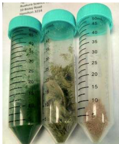
Figure 3: Biomass used for initial digestibility trials. The left most vial has the microalga, the right most vial the bacterium, and the centre vial has the two organisms grown together (co-cultured) in smaller lab photobioreactors (not shown).
