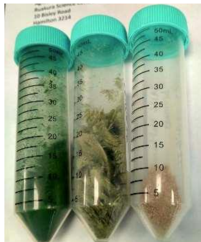
Figure 3: Biomass used for initial digestibility trials. The left most vial has the microalga, the right most vial the bacterium, and the centre vial has the two organisms grown together (co-cultured) in smaller lab bioreactors (not shown). The biomass ratio in the co-culture is approximately 1:1 (dry weight basis).
