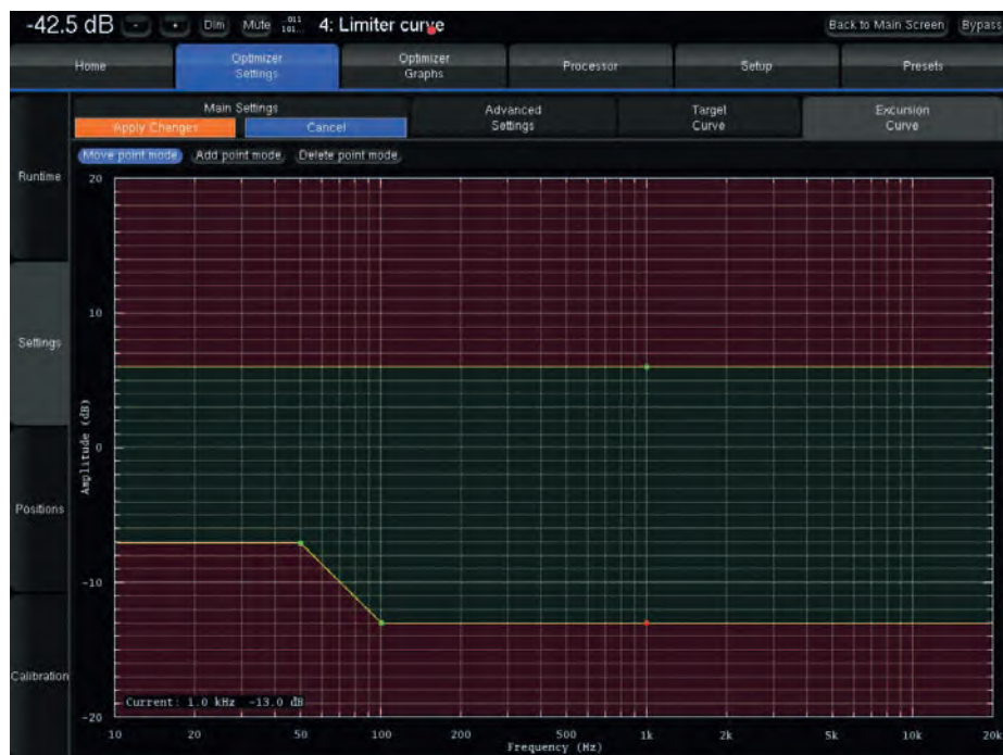
Figure 117: example of a limiter curve for maximum boost/attenuation
