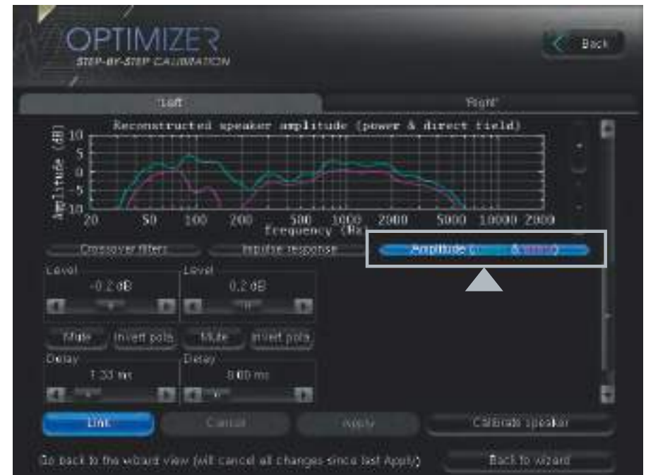
Amplitude (power & direct) response after calibration
