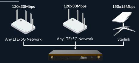
Multiple WAN bonding provides bandwidth up to ~390x80Mbps, while also providing carrier-redundancy for high uptime environments.
