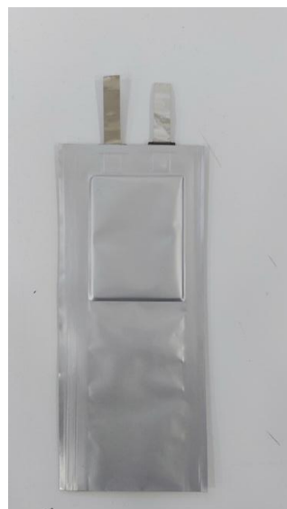
Figure 6.1. 300 mAh pouch cell charge-discharge test results (FRNC41 recycled cathode) with the digital image of the cell
