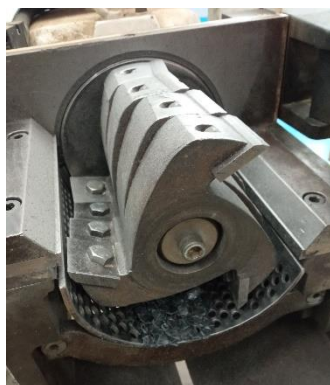
Figure 12. Shredder mill and shredder chamber.
