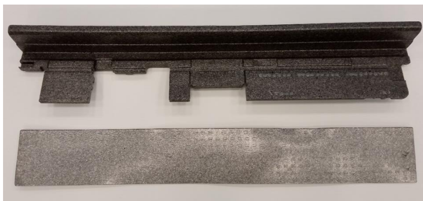
Figure 22. PP foamed extracted from EV battery pack.
