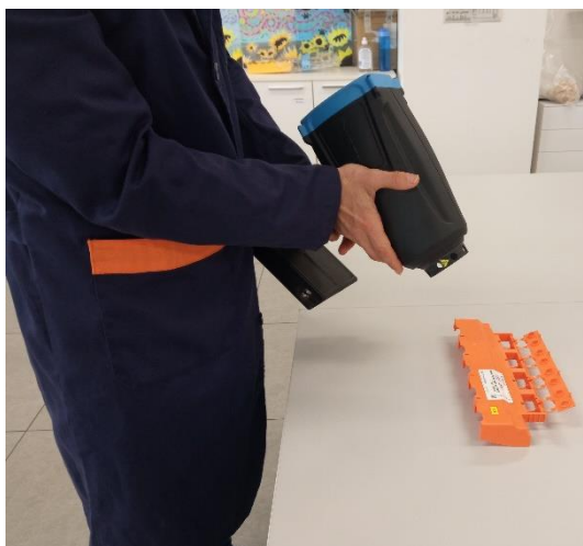
Figure 2. Polymer type identification with handheld NIR analyser.
