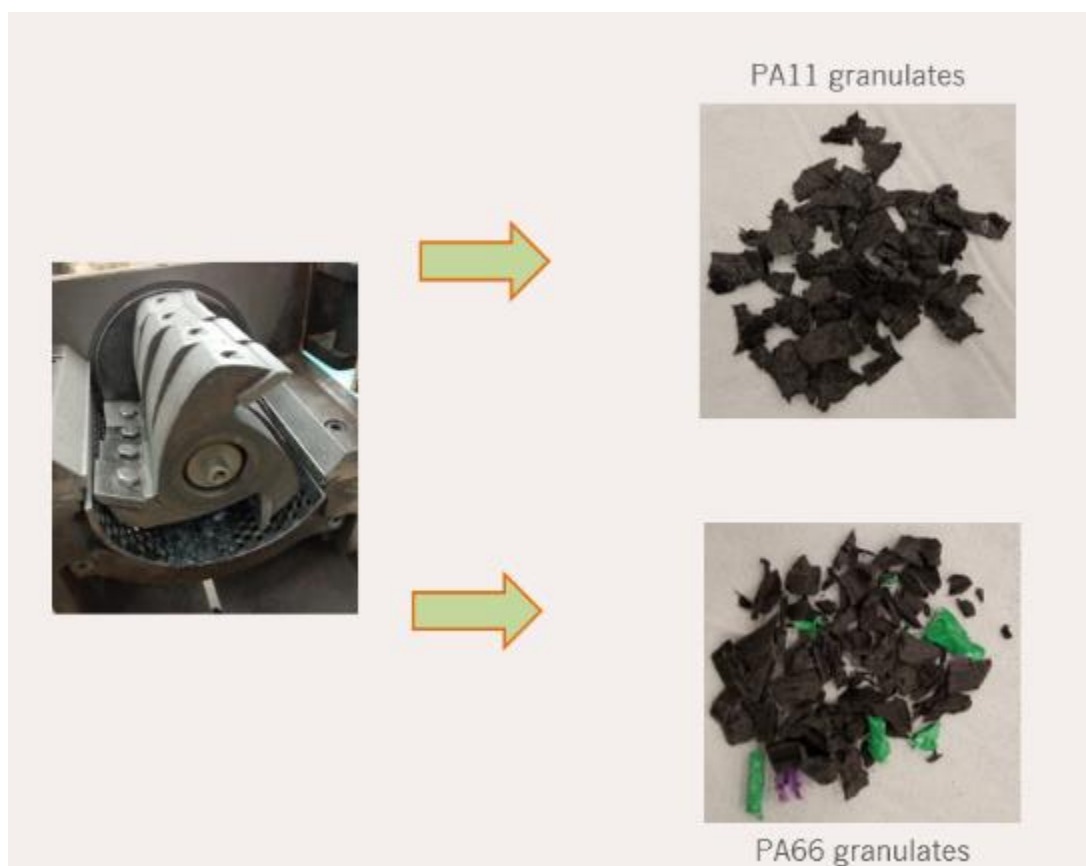
Figure 19. Thermoplastic granulates obtained after shredding.
