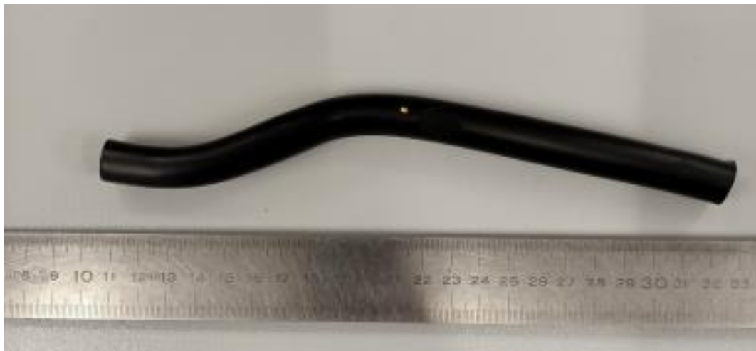
Figure 16. Pipes extracted from battery pack cooling system.
