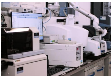
Figure 3. Polymer type identification in laboratory FTIR analyser.
