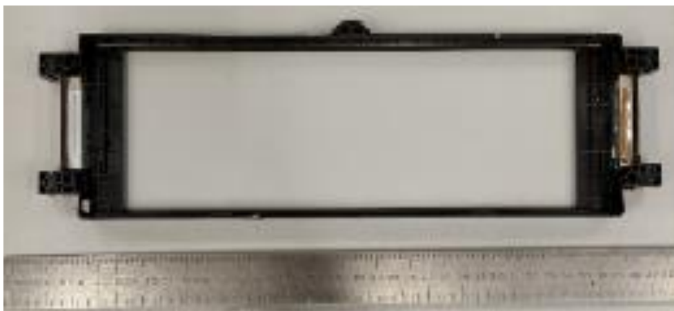
Figure 5. Cell pouch frames form battery modules.
