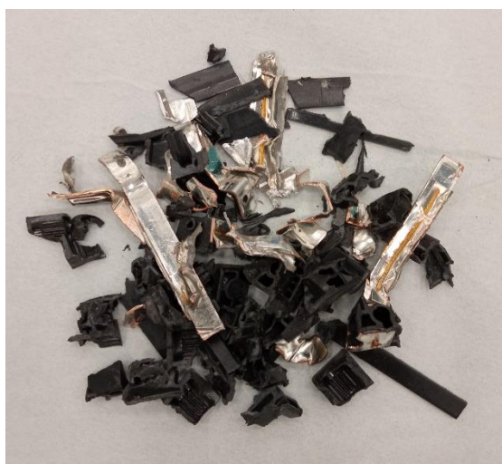
Figure 10. Mixed reduced parts after ferro-magnetic separation.
