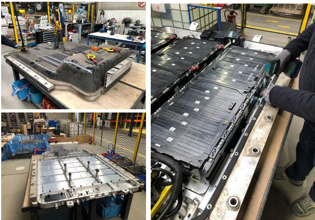
Figure 1. Original battery and different steps of its dismantling at Accurec.
