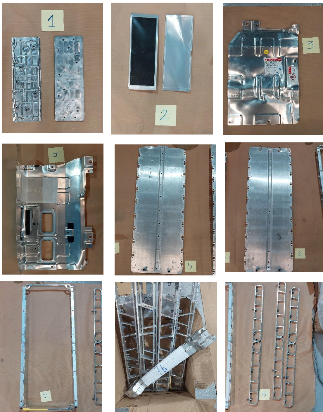
Figure 2. Classification of aluminium battery case parts a) module covers, b) separators, c) and d) case, e) and f) cooling floor, g), h) and i) frames.
