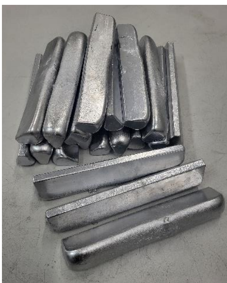
Figure 11. Billets of AlSi7Mg produced at EUT facilities.
