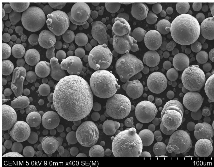
Figure 8. Scanning electron microscope image of the powder fraction < 63 \mu\text{m} .
