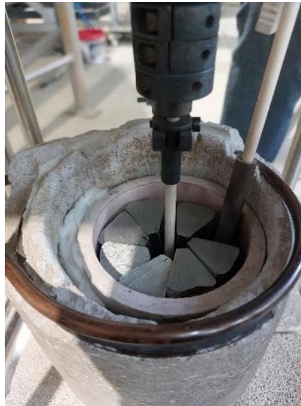
Figure 13. Alumina crucible filled with AlSi7Mg billets.
