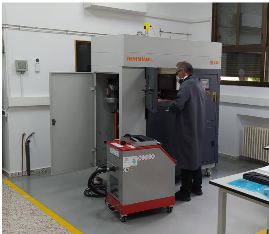
Figure 23. SLM equipment available at CSIC
