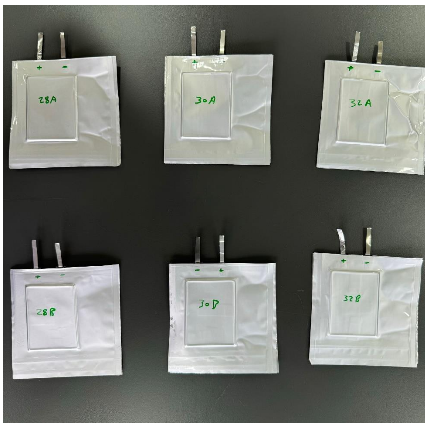
Figure 67. Digital images of assembled pouch cell assembled with recycled cathode materials.
