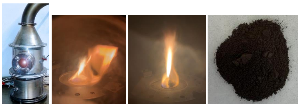
Figure 3. Laboratory FSP equipment, different flame morphologies and cathode powder collected.
