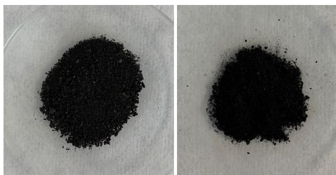
Figure 15. Optimized Li-NMC811 powder produced, 1) after light drying and 2) after thermal treatment.
