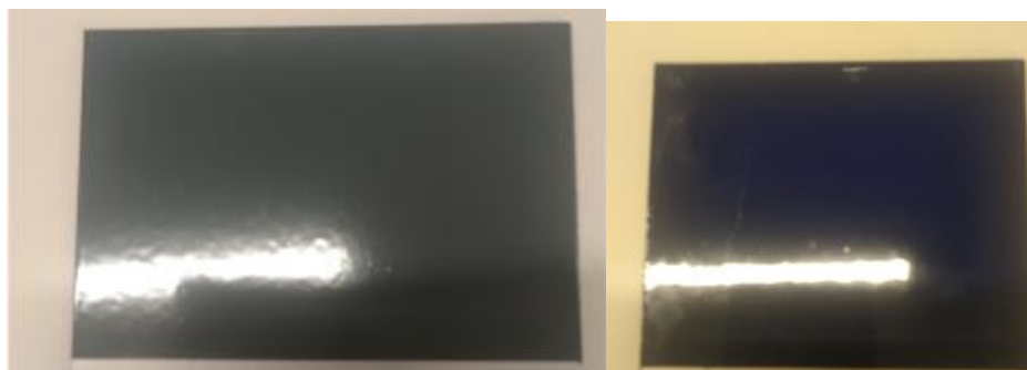
Figure 11 Enameled steel with frits (NiO bearing left).
