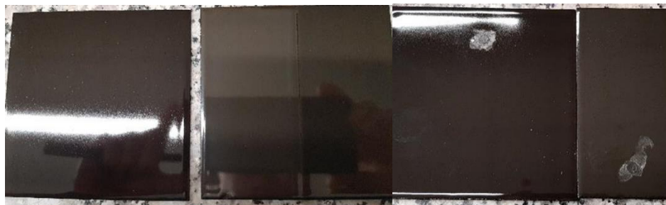
Figure 12 Left Steel enameled with std frit and novel frits std (left) 50% 100% replacement-Right adhesion test
