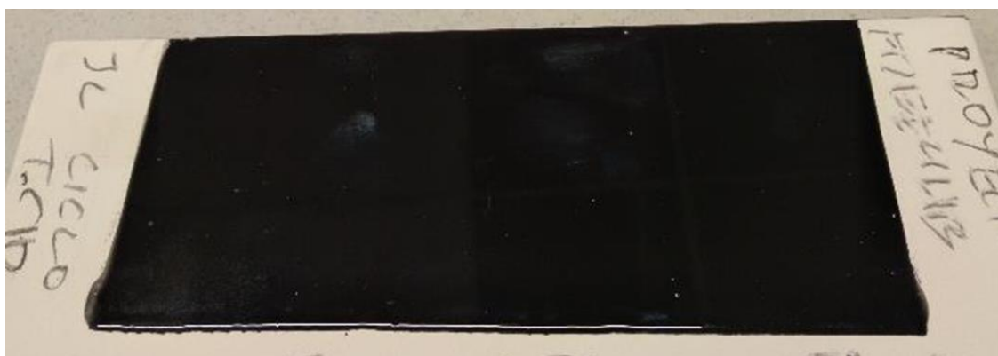
Figure 10 pigments in tile glaze (std-25 %replacement-10 % replacement)
