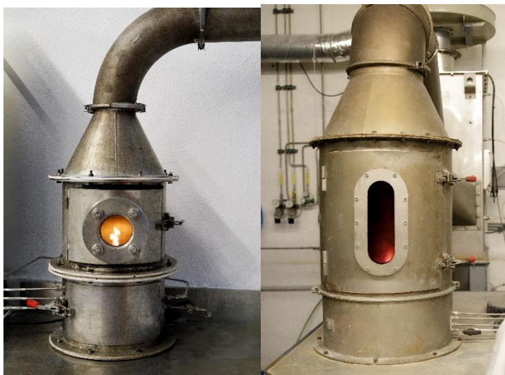
Figure 43. Left) Laboratory FSP equipment, 10g/h. Right) Pilot FSP equipment, 100g/h.
