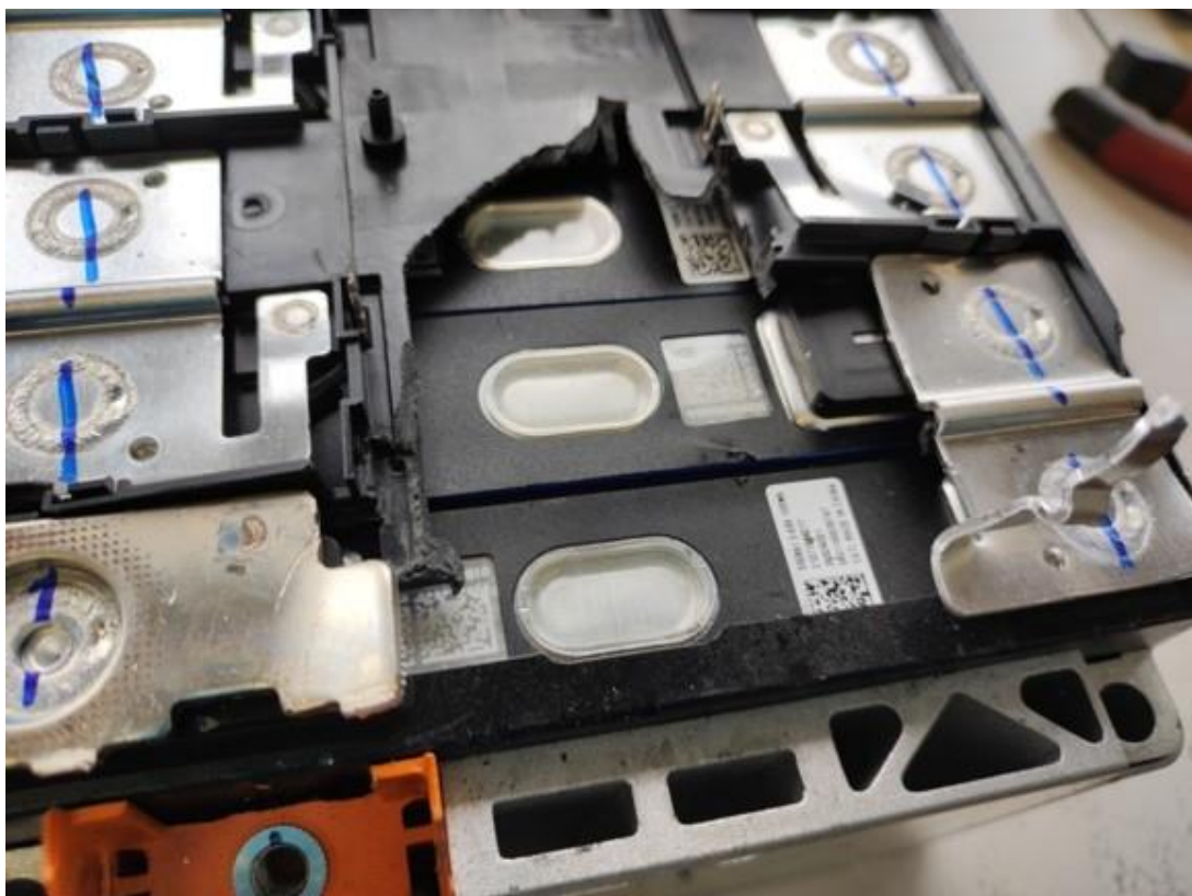
Figure 1. Hyundai Kona battery internal structure (l); Volkswagen module dismantling (r).
