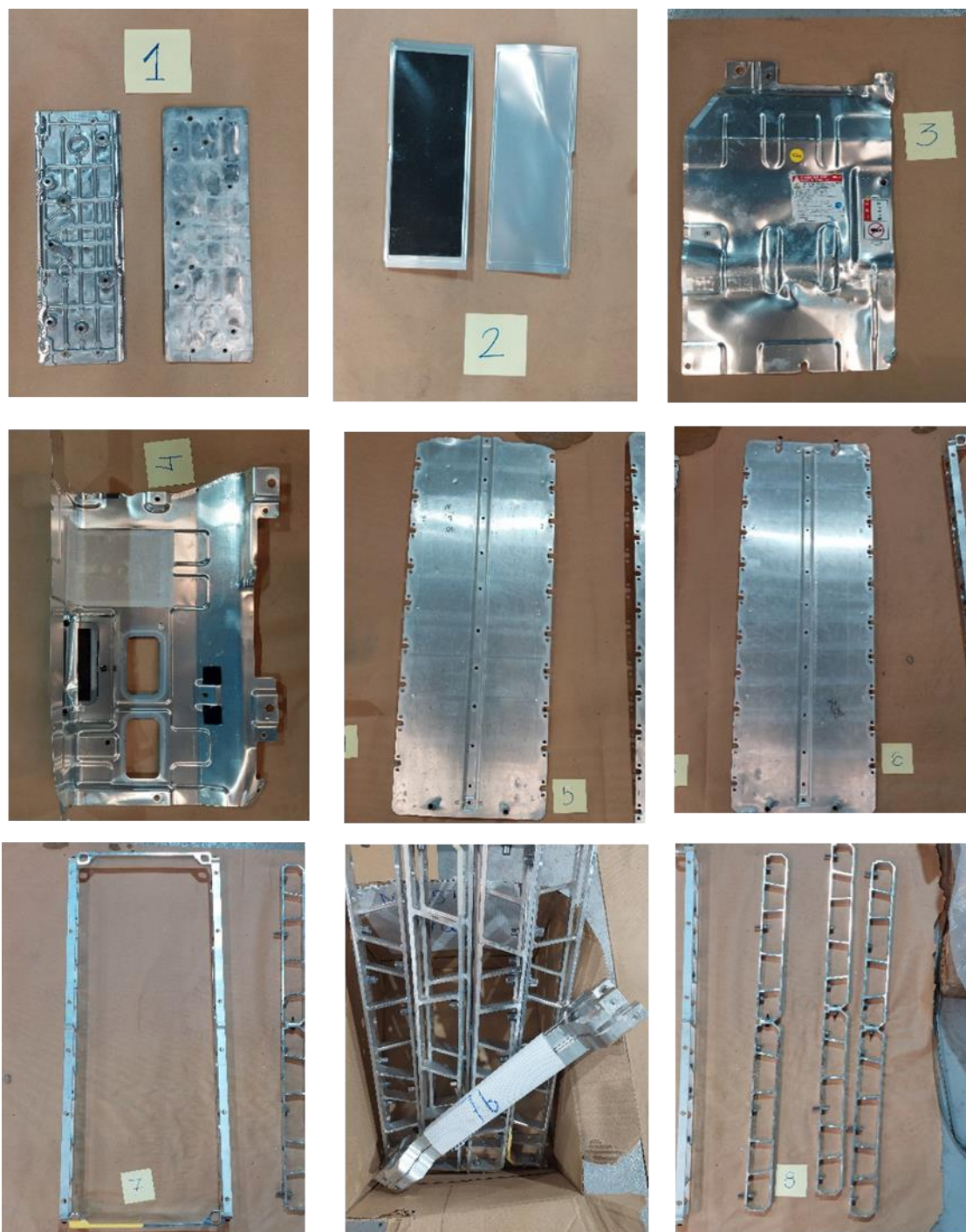
Figure 29. Classification of aluminium battery case parts a) module covers, b) separators, c) and d) case, e) and f) cooling floor, g), h) and i) frames.
