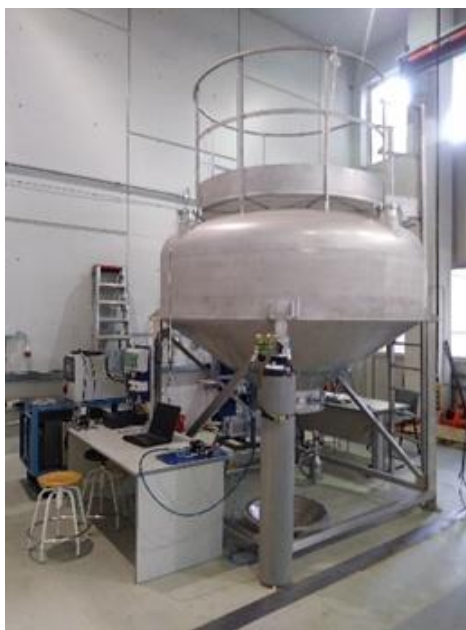
Figure 32. Centrifugal atomizer equipment used at Eurecat for the production of AlSi7Mg powder.
