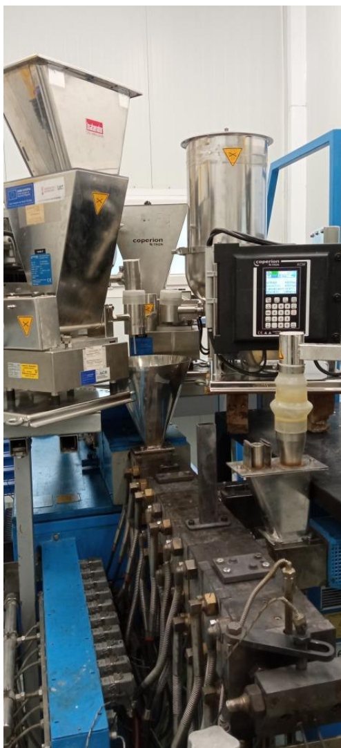
Figure 25. Extrusion compounding line in AIMPLAS pilot plant.
