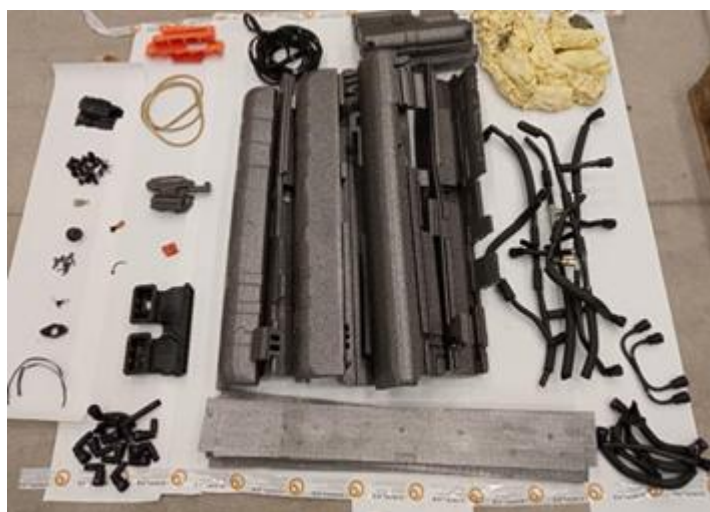
Figure 16. Plastic parts extracted from battery pack dismantling.
