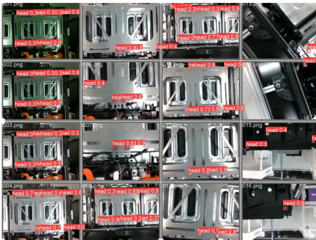
Image: Screw detection achieved training the model using YOLO.
