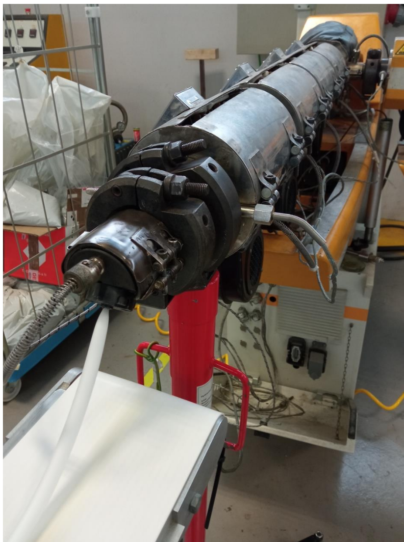
Figure 28. Foaming extrusion line in AIMPLAS pilot plant.
