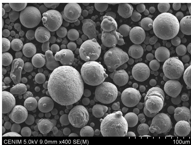
Figure 33. Scanning electron microscope image of the powder fraction < 63 \mu\text{m} obtained from VIGA atomisation
