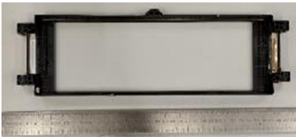
Figure 17. Cell pouch frames from battery modules.
