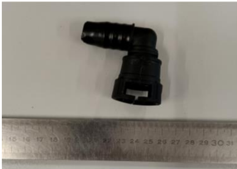
Figure 20. Fittings extracted from battery pack cooling system.
