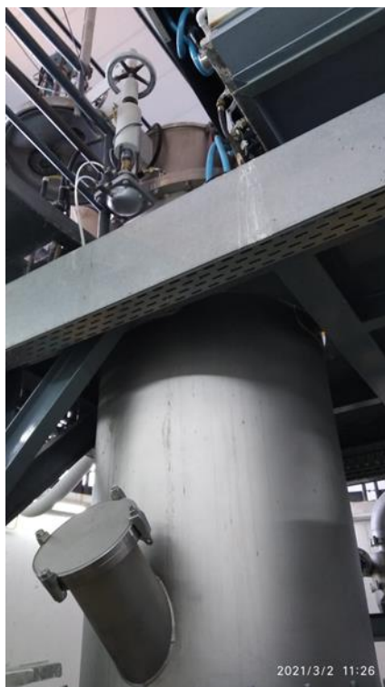
Figure 31. VIGA equipment used at the CSIC for the production of AlSi7 powder.
