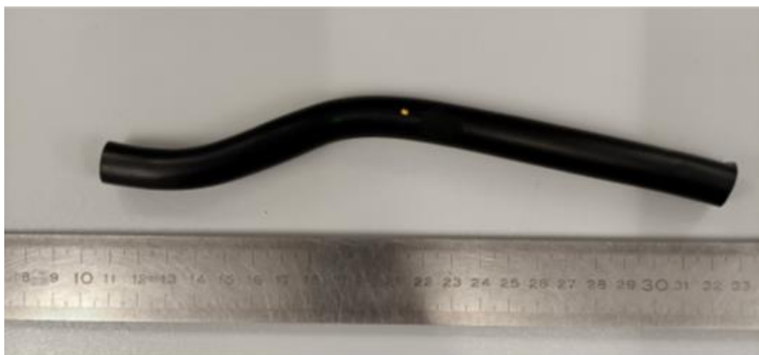
Figure 19. Pipes extracted from battery pack cooling system.
