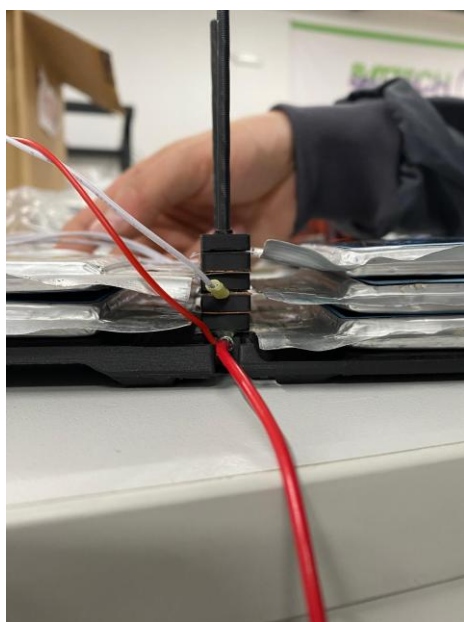
Figure 24. (Left) Side view of half of the cells already installed in the battery, along with their corresponding sensors. (Right) Five cells already mounted in the battery pack.
