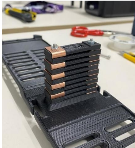
Figure 21. Contactor stacked with the contactor copper plate and secured in the lower frame.
