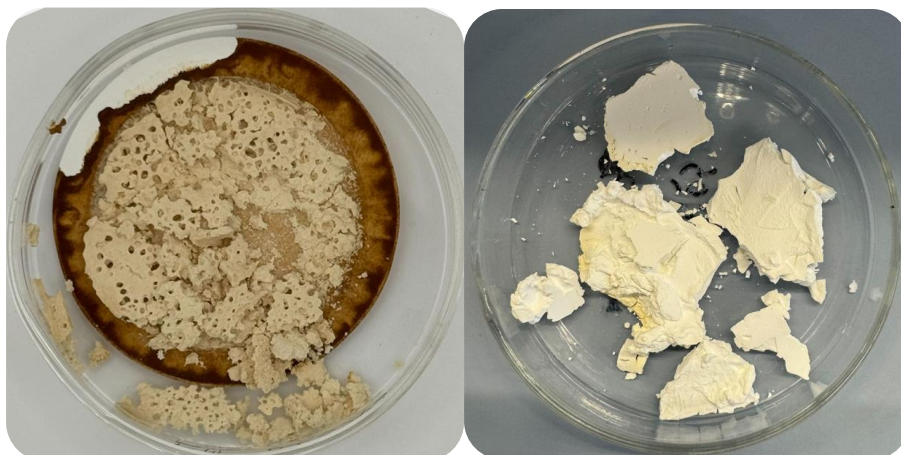
Figure 48. Lithium phosphate from NADES (left) and citric acid (right).
