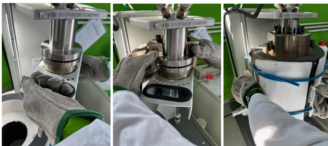
Figure 46. Hydrothermal re-lithiation beginning.
