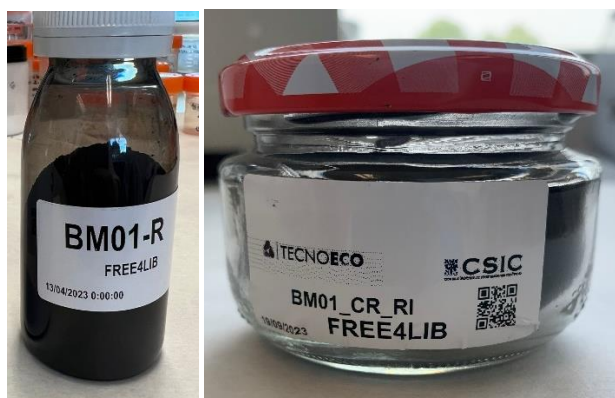
Figure 108. Residue from the leaching process.
