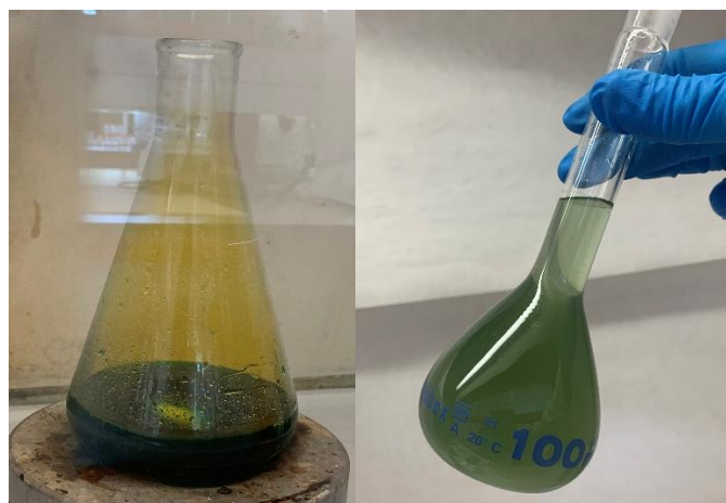
Figure 131. Optimised acid digestion of the cathode powder.
