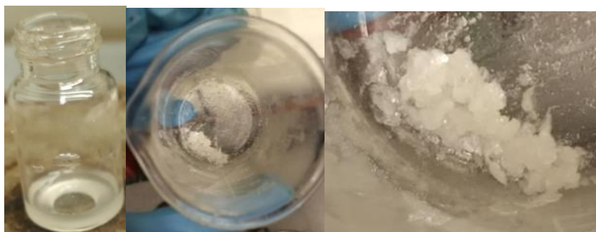
Figure 175. Lithium nitrate obtaining process from HNO 3 reaction.
