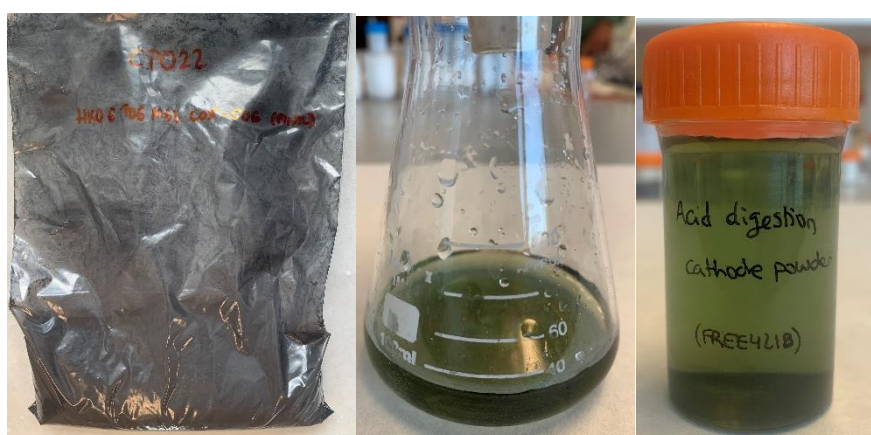
Figure 1012. Initial acid digestion of the cathode powder.
