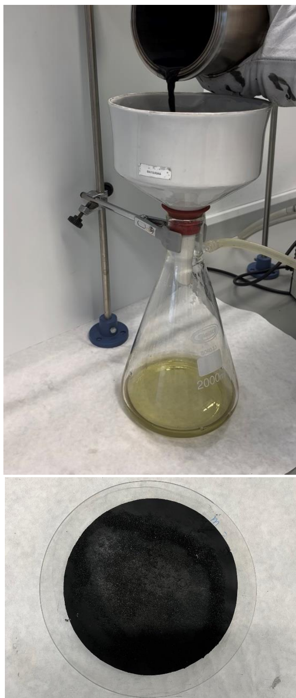
Figure 47. Filtered cathode material after hydrothermal re-lithiation.
