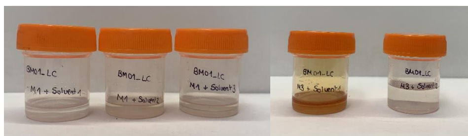
Figure 153. Solvent tests carried out with the lithium carbonate. Left) Two-phase solutions, Right) Homogeneous solutions.
