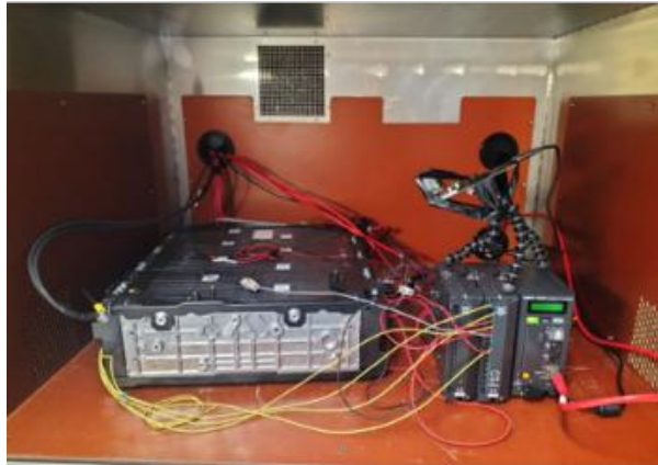
Figure 7: Hyundai Kona 9s3p module tested.
