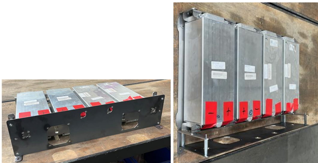
Figure 17. The manufacture sliders to be mounted in each rack of the BESS cabinet
