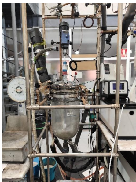
Figure 4. Glass reactor used in the leaching steps.
