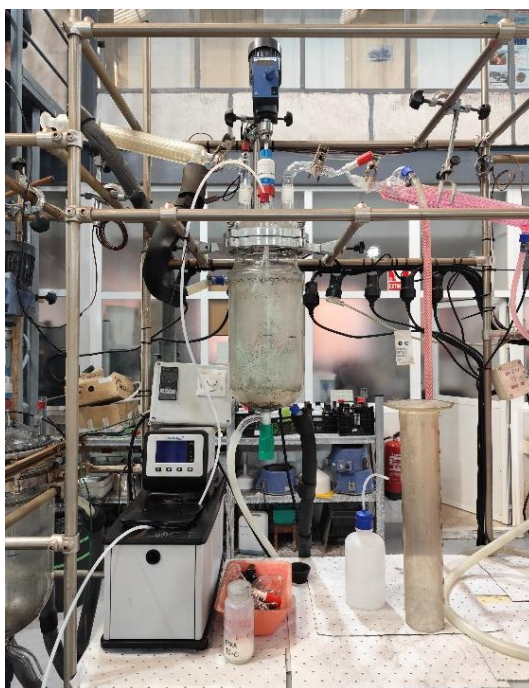
Figure 6 Precipitation reactor (obtention of PRE03, Co+Ni+Mn oxalate)
