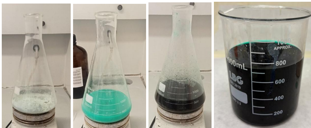
Figure 30. Evolution of the recycled powder during the acid digestion, and final solution.
