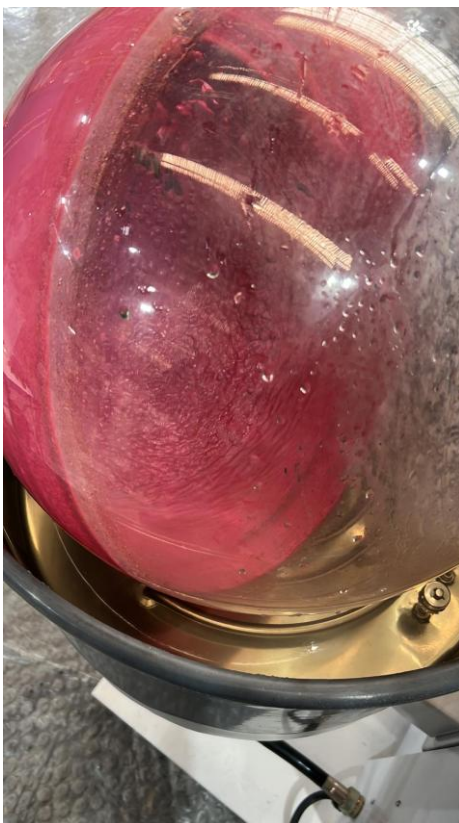
Figure 8. Rotavapor used in evaporative crystallization to obtain PRE04 and PRE05 (Ni+Mn oxalate and \text{CoSO}_4 ).
