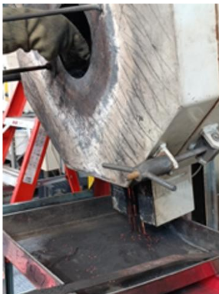
Figure 3. Furnace used for the carboreduction process.
