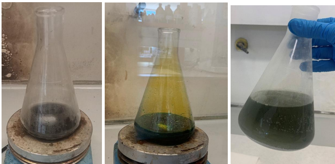
Figure 28. Acid digestion of recycled material from CARTIF.
