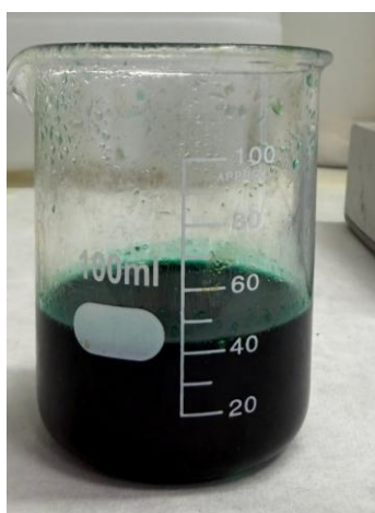
Figure 31. Liquid precursor mixture for LiNMC811.
