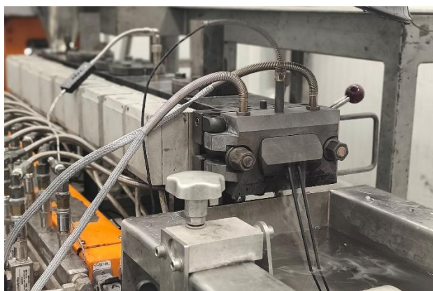
Figure 15. Upcycling process of decontaminated PA11 pellets via extrusion compounding.
