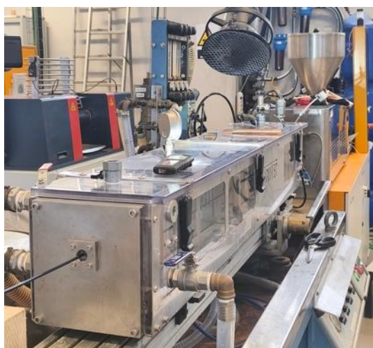
Figure 16. Piping extrusion line.
