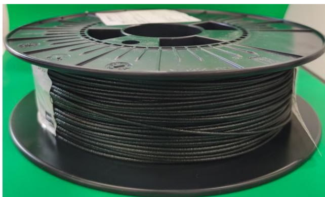
Figure 13. Filament 1,75 mm for 3D printing, made of 50% PCR PPE
