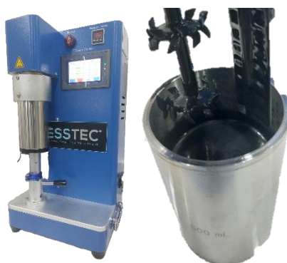
Figure 4.1 High shear, planetary vacuum mixing process.
