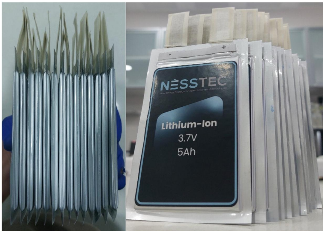
Figure 4.8 Aging, formation and electrochemical tests of produced pouch-cells.
