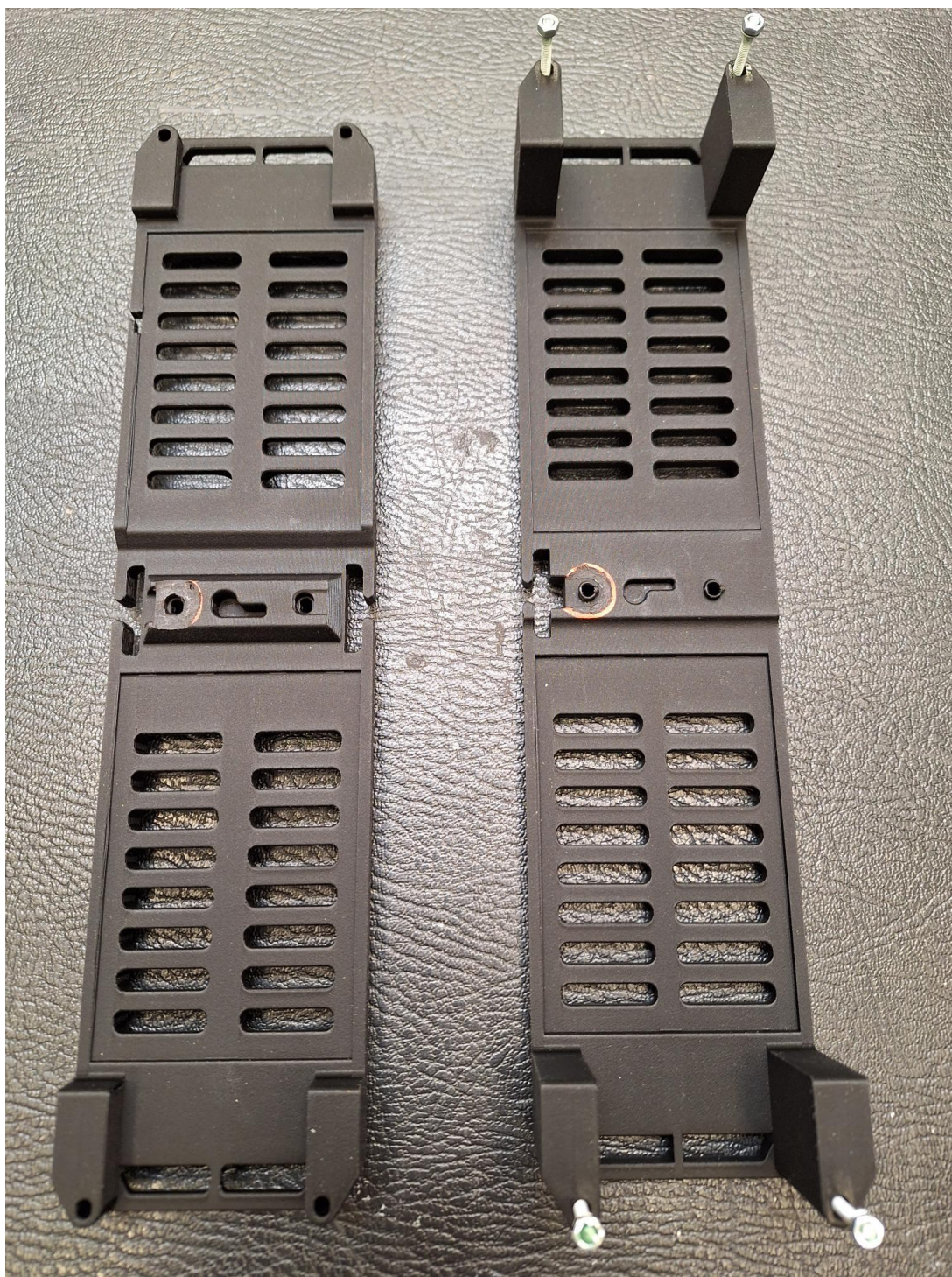
Figure 3 3D printed cell carrier
