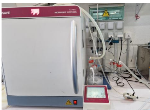
Figure 11. Microwave- assisted by pyrolysis set up.
