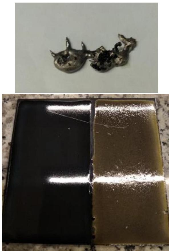
Figure 7. Reduced iron. Enamel performance. Left std, right using BM FIWKS
