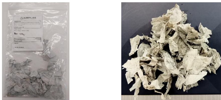
Figure 10. Thermoset sample recovered from EoL battery packs.
