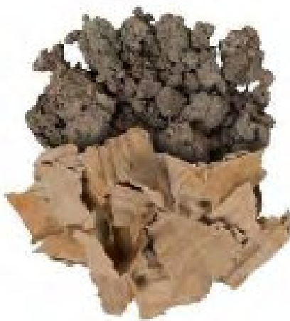
The images above show the three main stages of cellulose fibreboard making process. It starts with paper waste being shredded cellulose fibre, which is then mixed with water binder and fire retardant. Finally the mixture is compressed to form a compact solid board.
