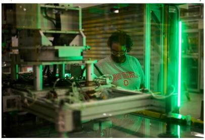
At a First Solar plant in Ohio, Rochelle Wilborn runs a test to ensure each panel has enough insulation to withstand high voltage.
