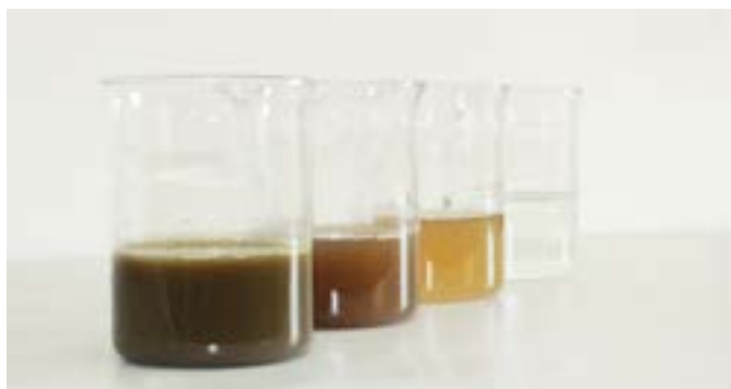
The solid matter of the liquid manure is separated from the water in four process steps. The result: Water, nutrient concentrate and dry fertilizer.
